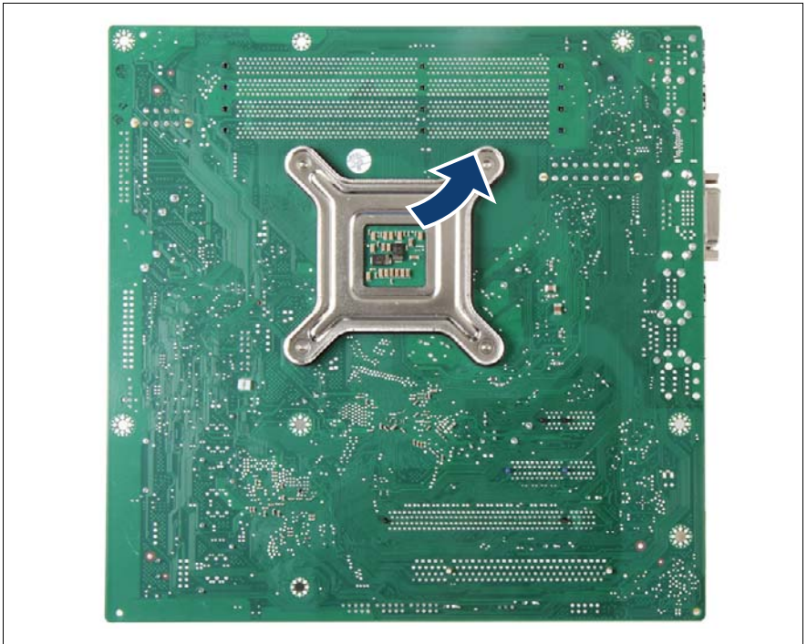
Figure 137: Removing the heat sink counter plate
